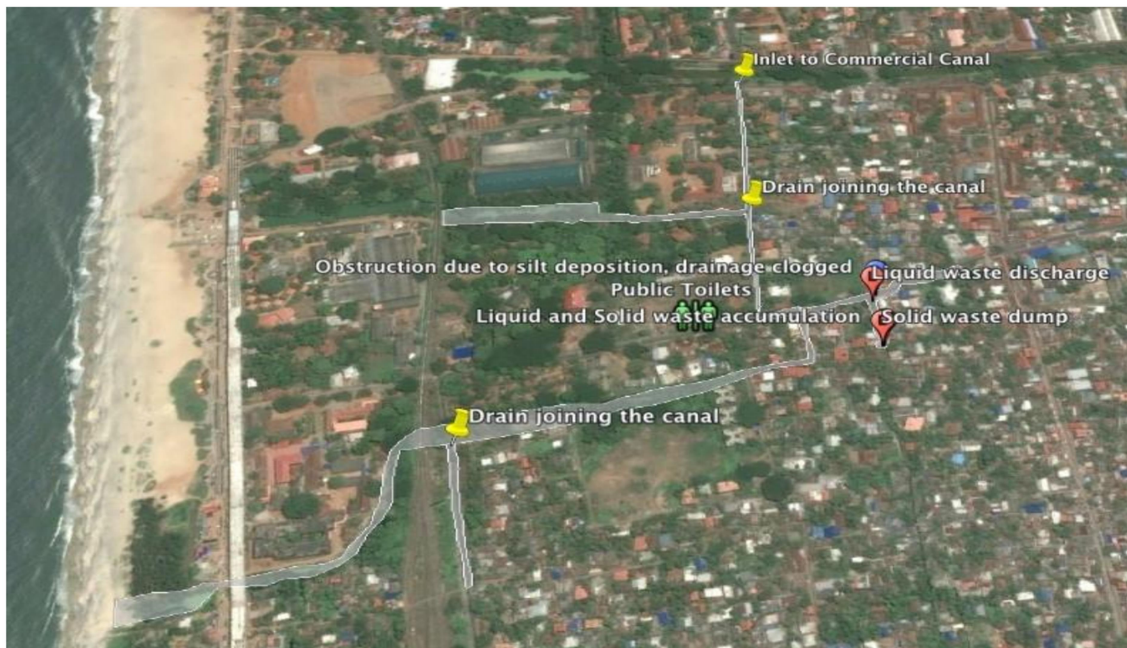
Figure 4 Drain mapping along Uppukuttipallam canal
